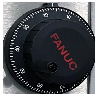
Figure 41 - MPG control wheel
