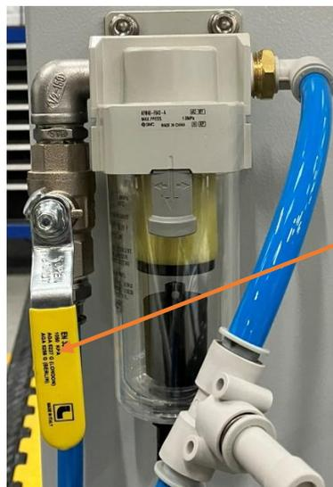
Main compressed air isolator valve to the machine (ON position)
