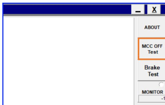
An **MCC off Test** of the safe stop function monitors the contact state of the electromagnetic contactor (MCC), compares the state with a command to the electromagnetic contactor, and checks that the safe stop function works normally. The Operator must carry out the test.
