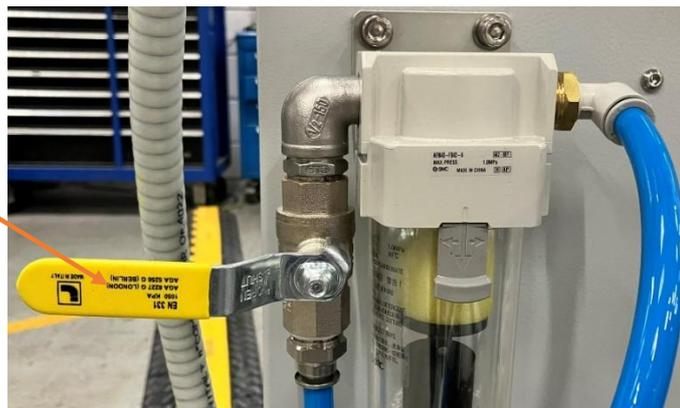
3. Disconnect the main air supply from the machine’s air supply feed pipe.
