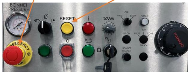
5. Once the “RESET” button has been pressed, perform a MCC test by pressing the “MCC OFF Test” button.
