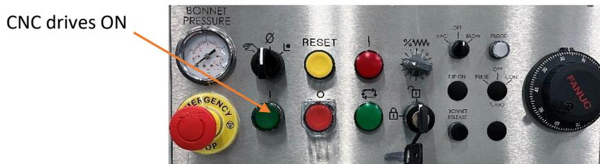
Figure 11 - CNC Drives ON switch
